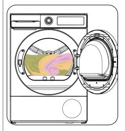
IMPORTANT: It is not recommended to load the dryer with more laundry than the amount shown in the figure. When overloaded, the drying performance of the dryer will decrease and the dryer and laundry might be damaged.
