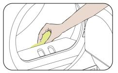
Inside the machine, there are humidity sensors that detect whether the laundry is dry or not.
